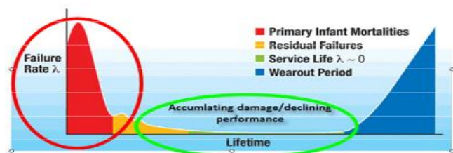
Figure 1 (a): Using Bathtub curve to explain PV Durability and Reliability Issues [4].
